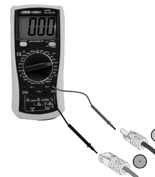
▲ Figure 4.6 PV+ Connector
